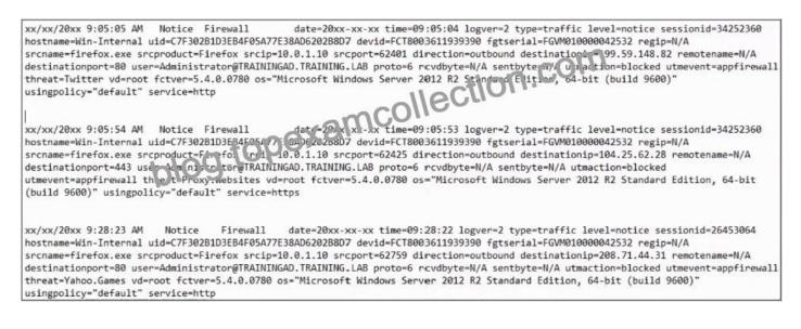
Based on the FortiClient logs shown in the exhibit which application is blocked by the application firewall?
